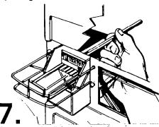
Secure coin slide mechanism from inside the control panel using the 3/16° bolt and wast included with the slide mechanism. Install coin box.
